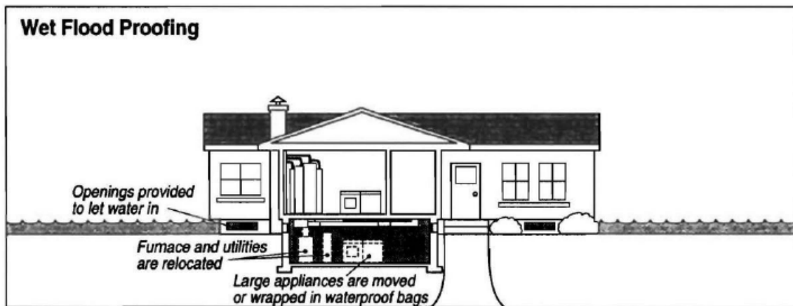
Figure 2. Nonstructural Wet Floodproofing Diagram
